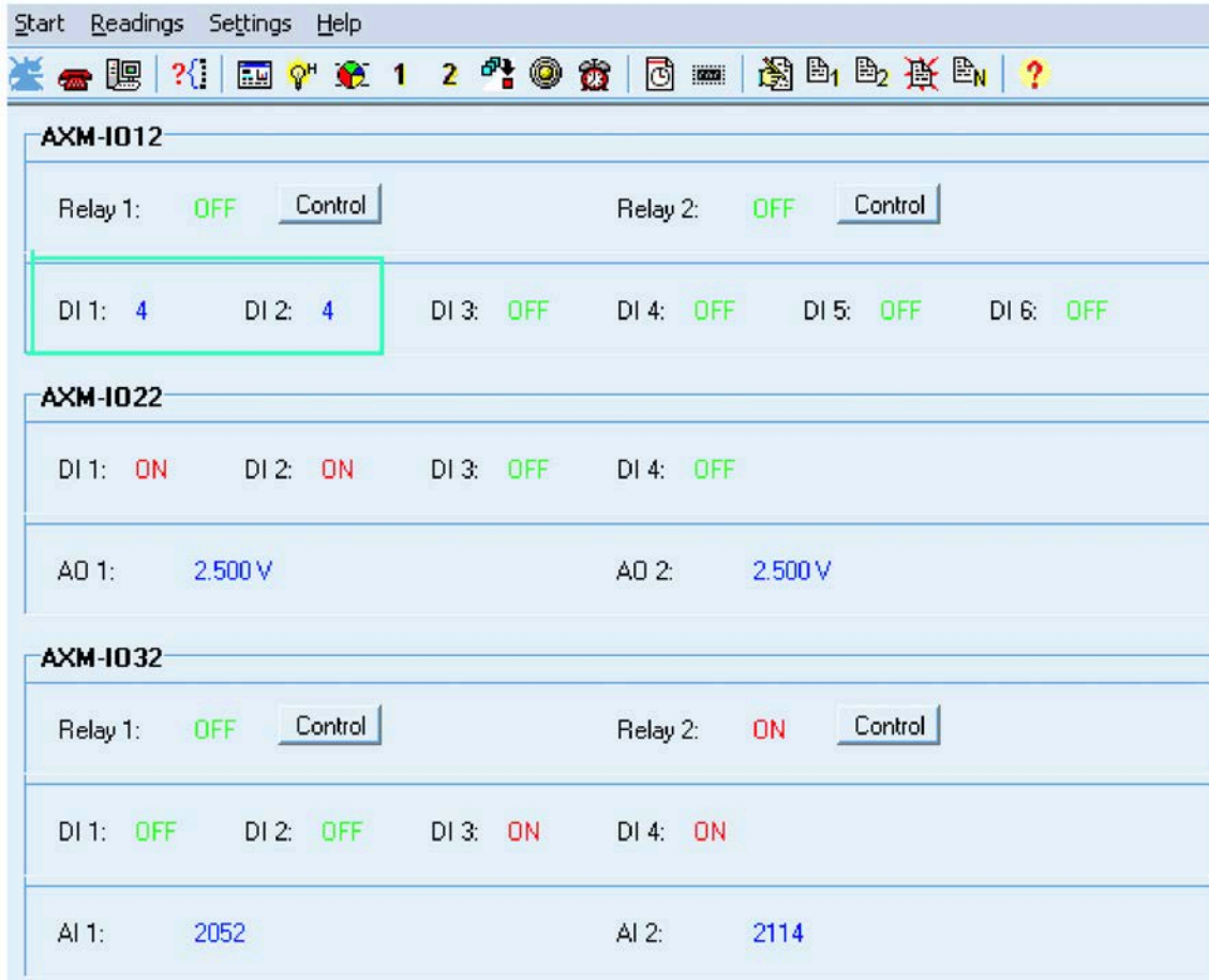
Fig 5-17 recorded number of pulses read by the utility software
