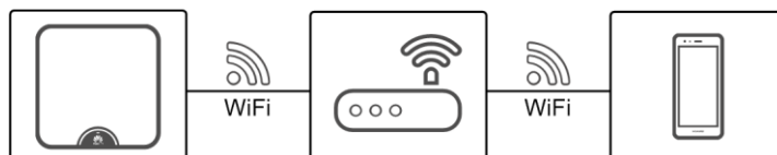
Figure 7-2 Mobile phone connecting to the SUN2000 over a router
