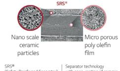
(Safety Reinforced Separator) with nano-coating of ceramic particles
