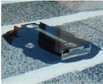
Test of water penetration on metal roof panel systems by static water pressure head.
