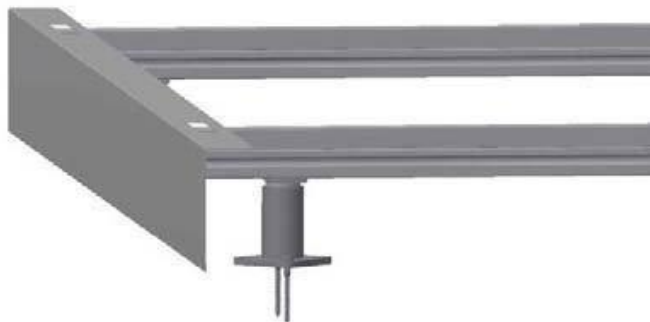
Position side fire flashings
