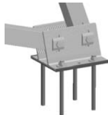
Rear: 4 Concrete anchors
