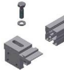
Connect KlickTop HB to S-5! U using M10 bolt and washer
