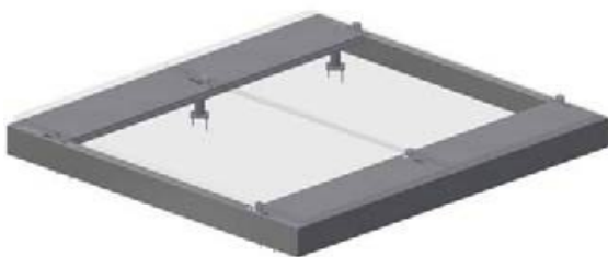
Position Modules; see page 14 for module installation instructions. Secure all connections using module clamps
