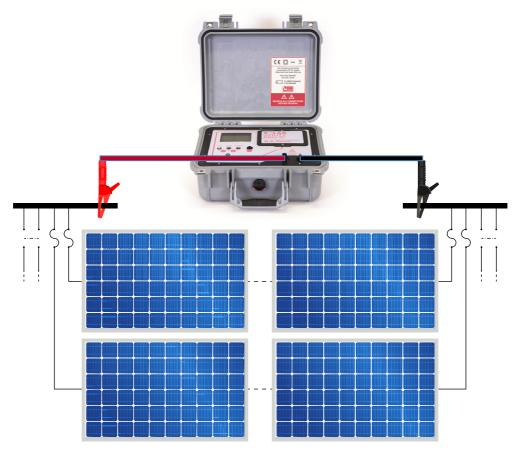
Connect the Solar Utility Pro securely to the PV module(s) or system as shown, using the supplied test leads.
