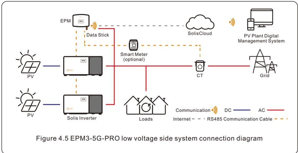
Figure 4.5 EPM3-5G-PRO low voltage side system connection diagram
