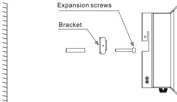
Figure 4.2 Fix the bracket on the wall
