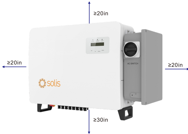
Figure 3.2 Clearance distances requirement for the inverter
